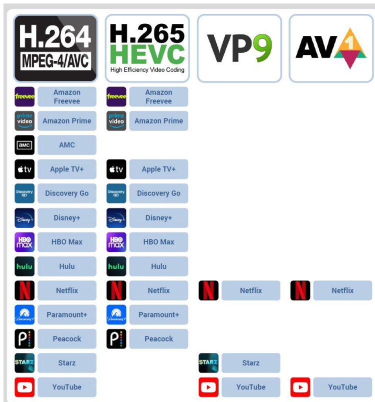
Figure 6. HEVC usage among prominent platforms in mid-2023.
