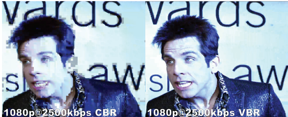
Figure 4-1. Sometimes CBR-encoded video exhibits transient quality glitches like this one in the movie Zoolander.
